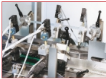
⑧ Four-gun gluing option ensures trays are sealed under all conditions.
