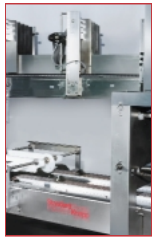
⑨ Stainless steel frame construction (optional) reduces machine maintenance requirements and allows for easy machine cleaning.
